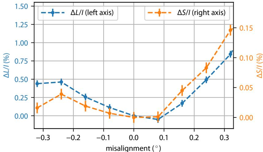
Figure 5: Misalignment of the polarimeter with respect to the light propagation axis cause systematic uncertainties in  $S/I$  (orange) and  $L/I$  (blue). This data was taken with a fixed incoming polarization of  $S/I = 16.3\%$  and  $L/I = 98.4\%$ .
