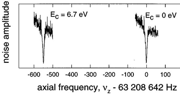
FIG. 16. Axial resonance of a single trapped electron (noise-shorting dip to the right) is shifted to a lower frequency (left) when the electron's cyclotron motion is excited to an energy of  $E_c = 6.7$  eV. When the cyclotron drive is turned off, the dip shifts back as the electron damps via its coupling to the radiation field in the trap cavity.
