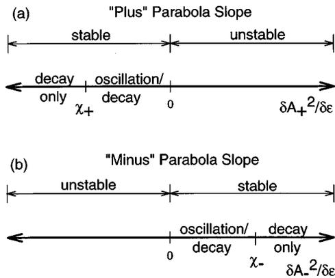
FIG. 14. Stability regions for each of the two steady state branches, as determined by  $\tau_2$  given in Eq. (17). The “plus” parabola [corresponding to  $\cos(\Psi_{ss})$  positive] must have a negative slope to be stable [shown in (a)]. The “minus” parabola [corresponding to  $\cos(\Psi_{ss})$  negative] must have a positive slope to be stable [shown in (b)]. The oscillatory regions, delineated by  $\chi_{\pm} = -4\epsilon_{\pm}A_{\pm}^2/(\gamma_z/2)^2$ , are discussed in the text.
