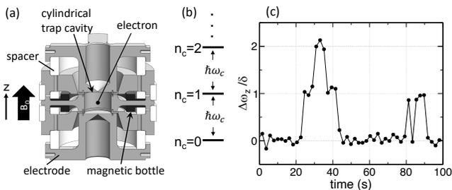
FIG. 1. (a) Single isolated electron in a cylindrical Penning trap. (b) Quantum cyclotron energy levels of the trapped electron. (c) Resolution of cyclotron states  $n_c$  by measuring axial frequency shift. A resonant external cyclotron excitation drive is applied.
