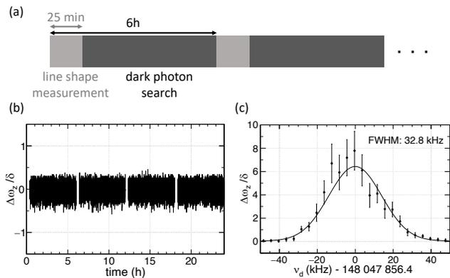
FIG. 4. (a) The DPDM measurement cycle. (b) Monitored axial frequency shift shows no DPDM-induced cyclotron excitations during 24 hours of the 7.4 day search. (c) Measured cyclotron line shape  $\chi(\omega, \omega_c)$  with the self-excitation on.
