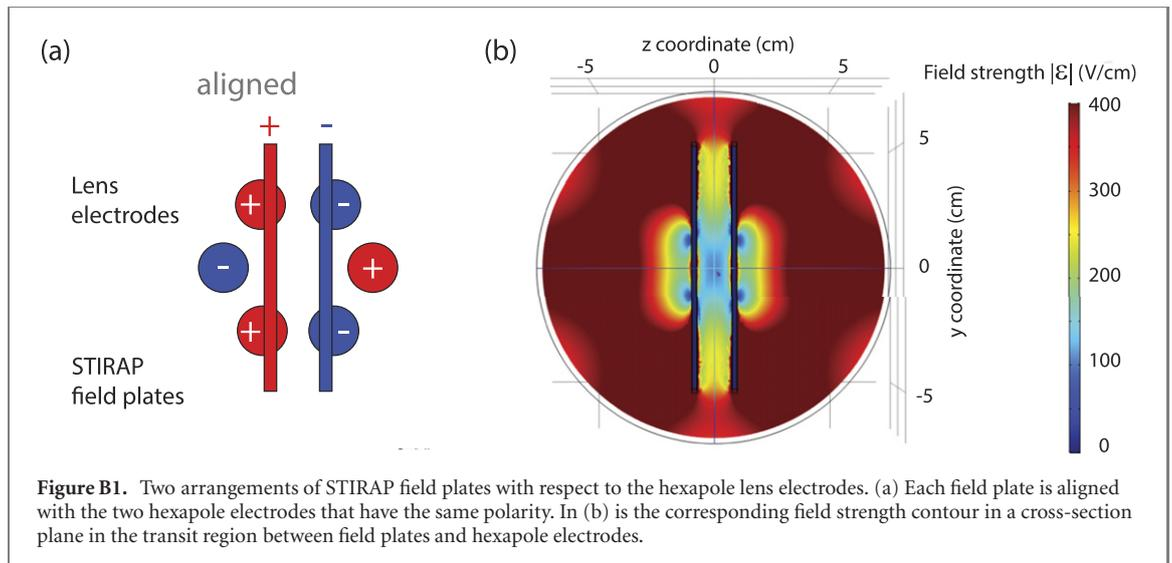
**Figure B1.** Two arrangements of STIRAP field plates with respect to the hexapole lens electrodes. (a) Each field plate is aligned with the two hexapole electrodes that have the same polarity. In (b) is the corresponding field strength contour in a cross-section plane in the transit region between field plates and hexapole electrodes.
