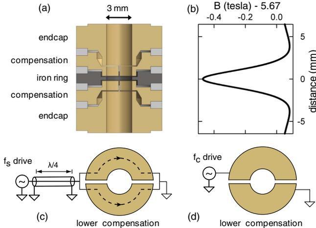
FIG. 2 (color online). (a) Electrodes of the analysis trap (cutaway side view) are copper with an iron ring. (b) The iron ring significantly alters  $B$  on axis. (c) Top view of the paths of the oscillating current for the spin flip drive. (d) An oscillating electric field (top view) drives  $\bar{p}$  cyclotron motion.
