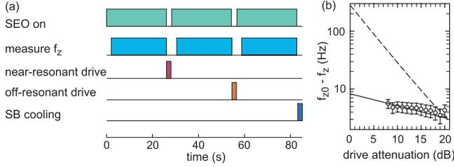
FIG. 3 (color online). (a) Spin measurement cycle. (b) The power shift in  $f_z$  due to the spin flip drive (points) is lower than was observed for the proton measurement with no transmission line transformer (dashes).
