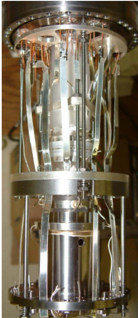
Figure 3.8: Photograph of planar Penning trap bolted below the LeptonCPT experiment. Electrical connections are made between electrodes and FEPs and the hermetically-sealed electrical feedthroughs of the pinbase via high-purity silver straps.
