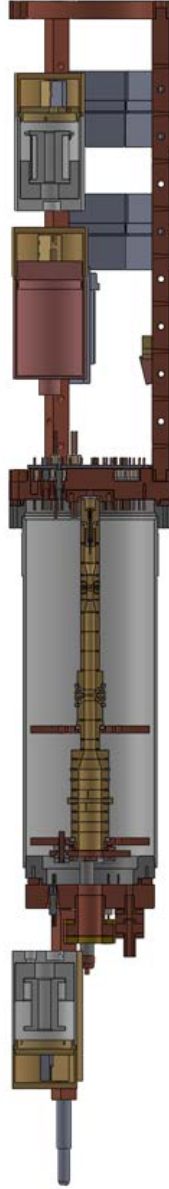
Figure 8.9: CAD model of tripod and trapcan with electronics and trap electrodes.
