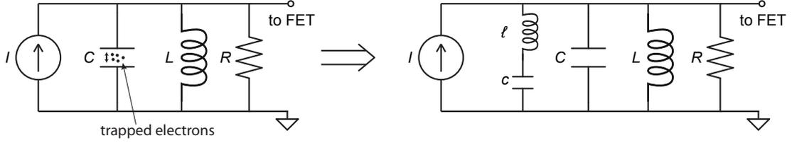
Figure 5.7: Series LC circuit representation of the trapped electrons in the RLC amplifier circuit.  $C$  is the trap capacitance,  $L$  is the inductance of the coaxial resonator,  $\ell$  and  $c$  represent the trapped particles and  $R$  is the effective resistance.
