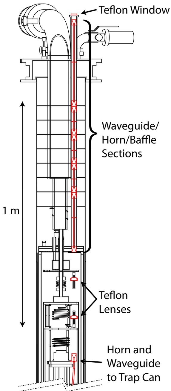
Figure 5.14: The microwave path from the top of the dilution refrigerator (300 K) to the horn at the mixing chamber (100 mK) is shown in red.
