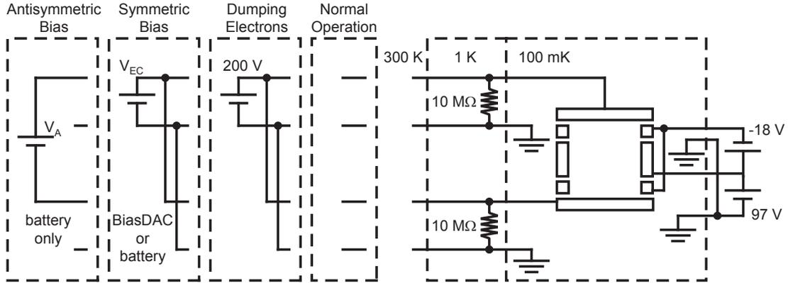
Figure 5.2: Typical endcap bias configurations. Note that the voltages shown here are for electrons. For positrons, the voltages would all have the opposite sign.
