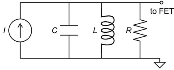
Figure 5.3: Parallel circuit representation of the input to the first stage amplifier.  $C$  is the trap capacitance,  $L$  is the inductance of the coaxial resonator and  $R$  is the effective resistance.
