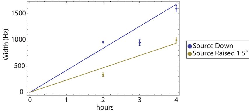
Figure 6.13: Raising the source 1.5 in above the usual loading position decreases the loading rate by nearly a factor of 2. These data were taken in configuration B in Fig. 6.9 and without firing the FEP beforehand.
