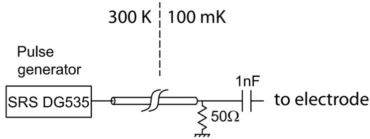
Figure 7.1: This is the basic pulsing scheme we plan to use to pulse positrons from the loading trap to the precision trap. This design is based on the circuit used in [99].
