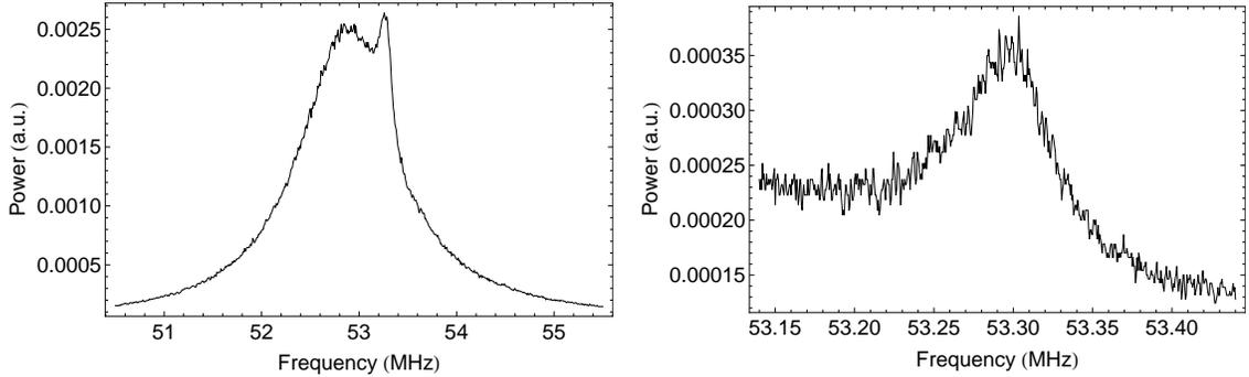
Figure 6.5: Typical loading trap amplifier noise resonances taken at 4K, showing the first stage on top of the second stage (left) and just the first stage (right). The first stage fits to  $Q \approx 800$ .
