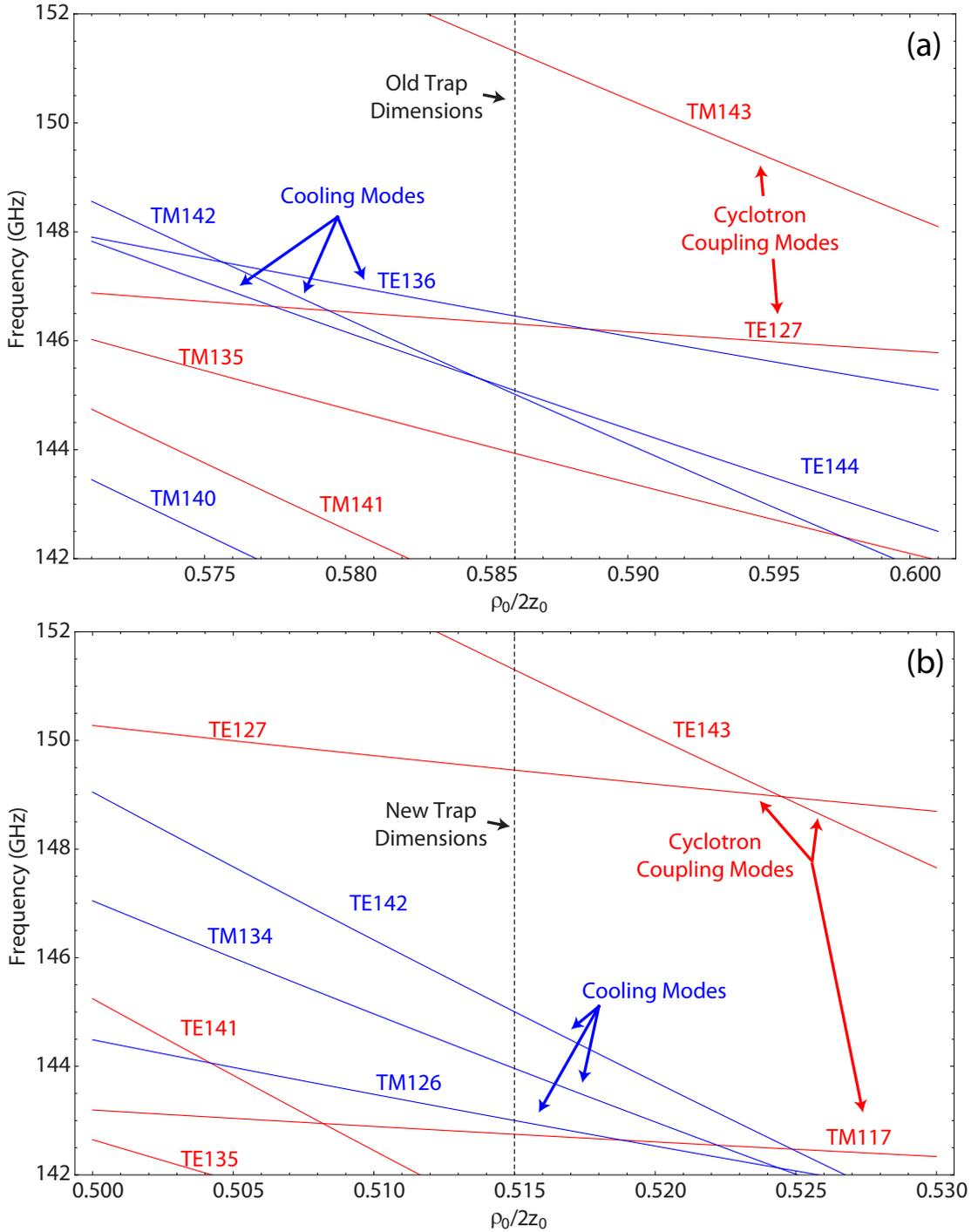
Figure 2.3: A comparison of the approximate cavity mode locations for different ratios of trap radius  $\rho_0$  to height  $2z_0$ . The modes in the trap used in the 2008 measurement are shown in (a) and those in the new precision trap are shown in (b).
