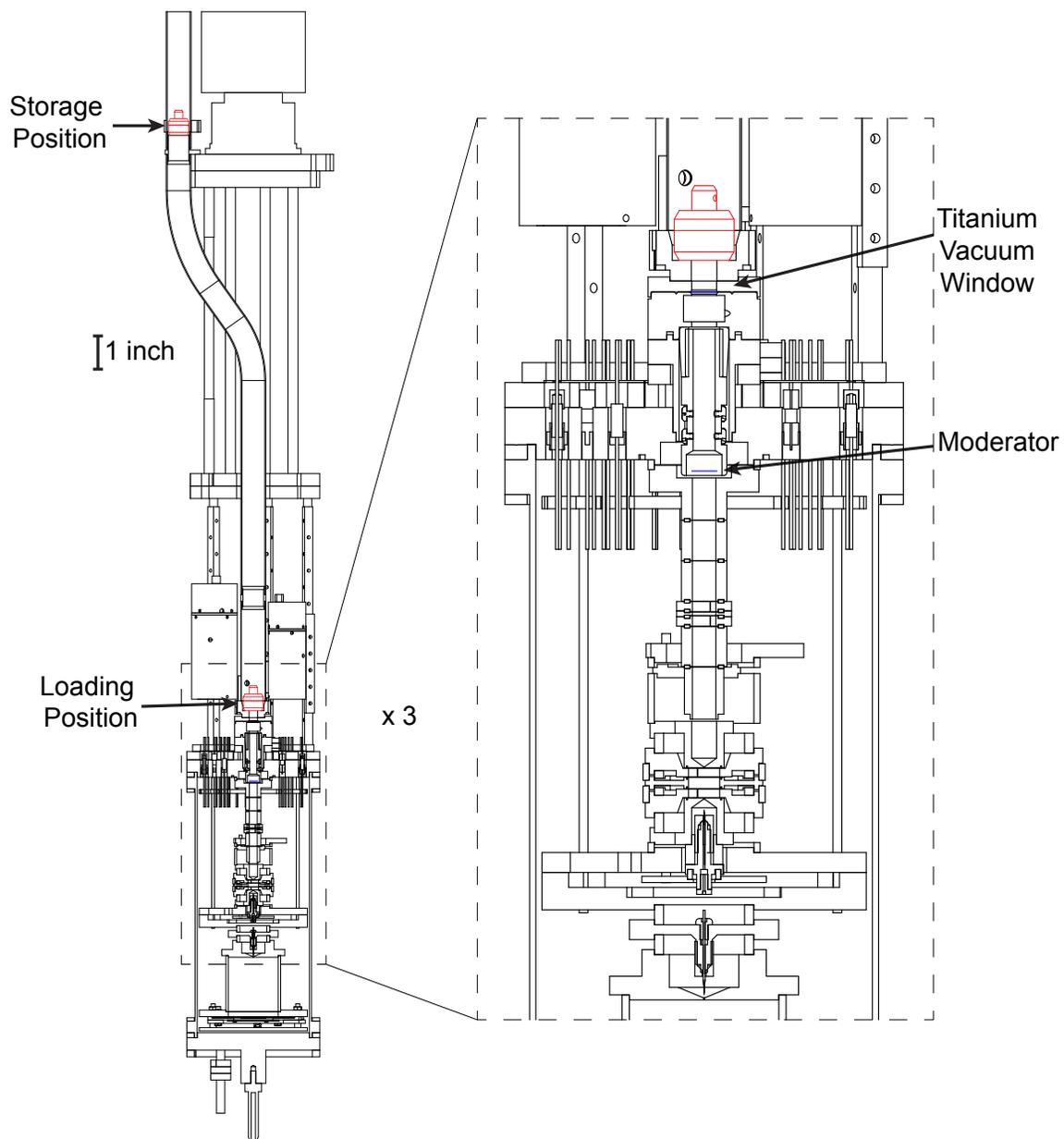
Figure 4.4: Positron source storage and loading positions
