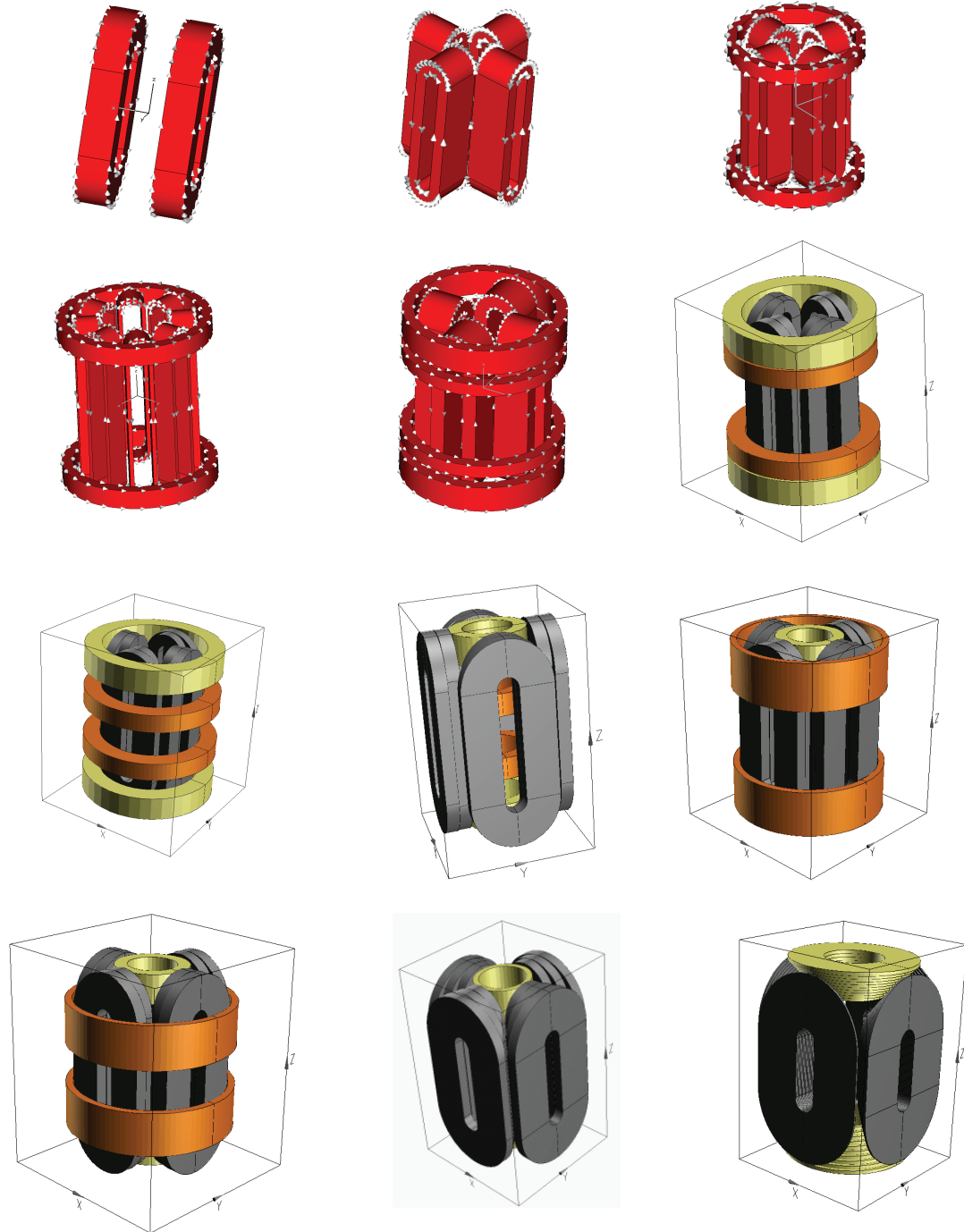
Figure 9.4: Coil designs considered for BTRAP Ioffe trap configuration. The yellow coils provide a field in the direction of the axial field of the penning trap, the orange coils oppose it in order to increase the trap depth.
