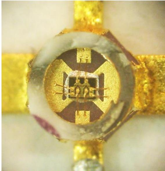
Figure 4.1: Fujitsu FHX13LG HEMT with the ceramic cover removed. The gate lead is at the bottom, the drain is at the top, and the side leads are both connected to the source. Carriers in the channel are conducted in the vertical direction.
