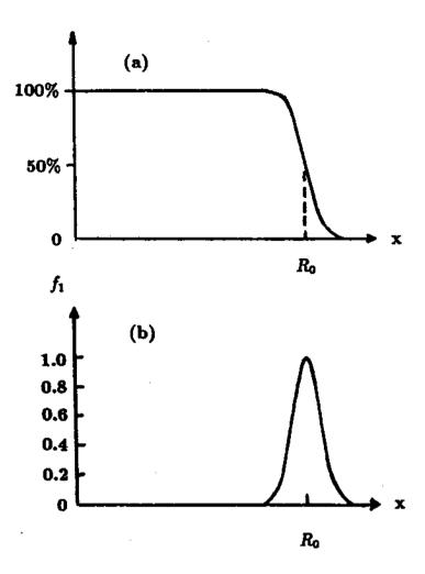
Figure 2.3: (a) An idealized range curve showing the fraction of particles in a beam penetrating to a given depth x. The mean range  $R_0$  is the point passed by half the particles. (b) The relative distribution of particles near mean range.
