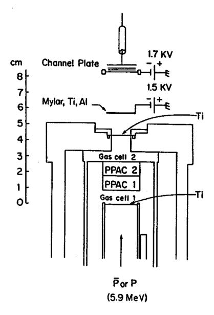
Figure 2.5: Time-of-flight apparatus. The apparatus from below 5 cm on the vertical scale remained in place for trapping experiments so that the incident antiprotons could be monitored and their energy tuned slightly. PPAC is the parallel plate avalanche counter.
