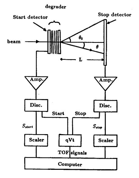
Figure 2.4: Transmission method for range curve and energy distribution measurements.
