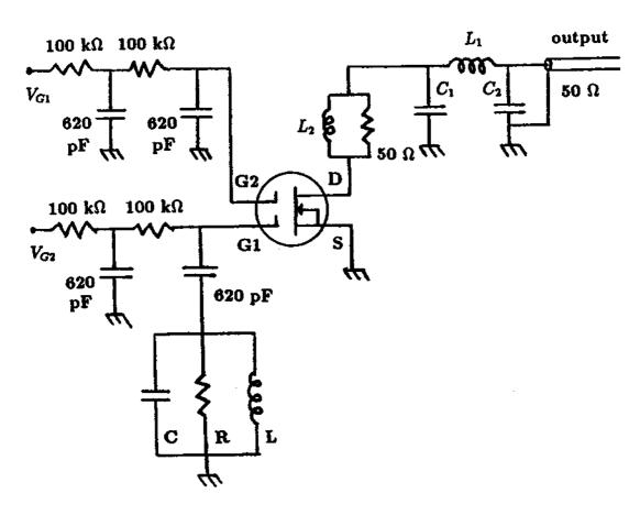
Figure 5.6: Dual-gate GaAs FET amplifier circuit.
