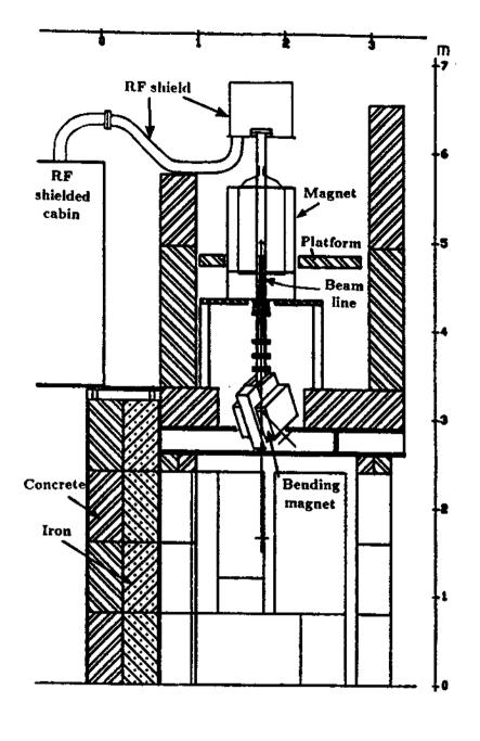
Figure 2.2: The zone layout of the TRAP experiment (PS196).
