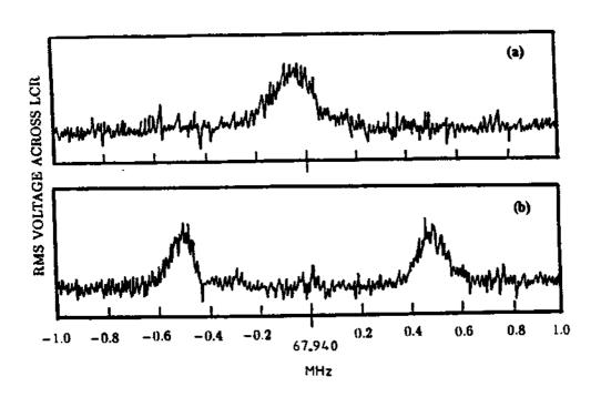
Figure 5.7: (a) Typical noise resonance for the LCR circuit at LHe temperature. (b) Modified signal when large electron cloud is present. The spacing of the two peaks of 1 MHz indicates that  $6 \times 10^6$  electrons are in the trap.
