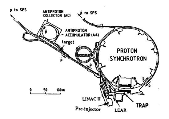
Figure 2.1: CERN facility for producing, transferring, storing and cooling antiprotons.
