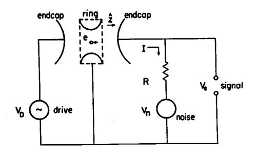
Figure 5.8: Detection and resistor damping of ion motion (from Ref. [73]).
