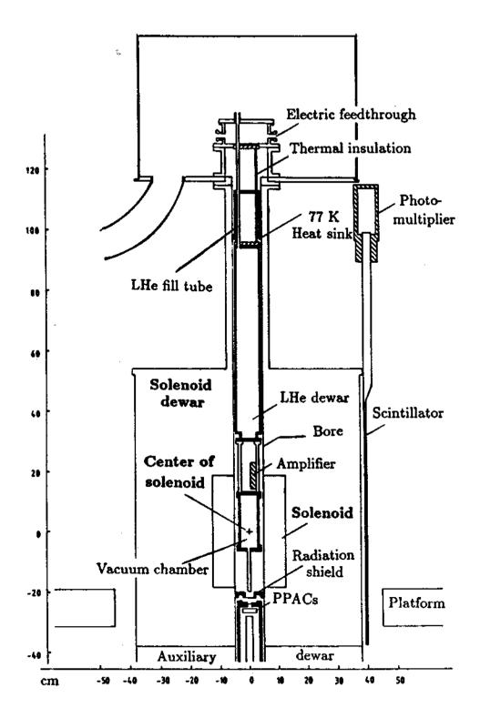
Figure 3.3: The apparatus for the antiproton trapping experiment.
