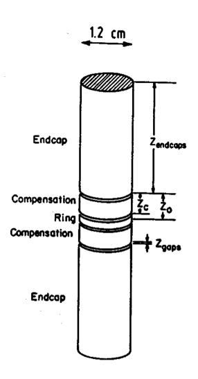
Figure 5.4: The cylindrical open-endcap ion trap (From Ref. [54]).
