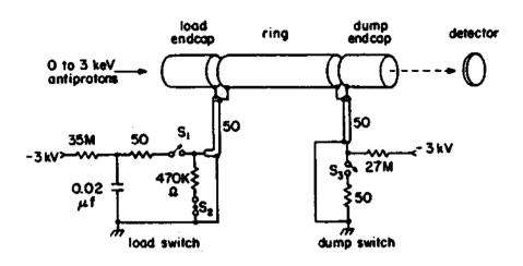
Figure 4.1: Simplified outline of the Penning trap electrodes and the idealized high-voltage switches used to capture antiprotons in flight.
