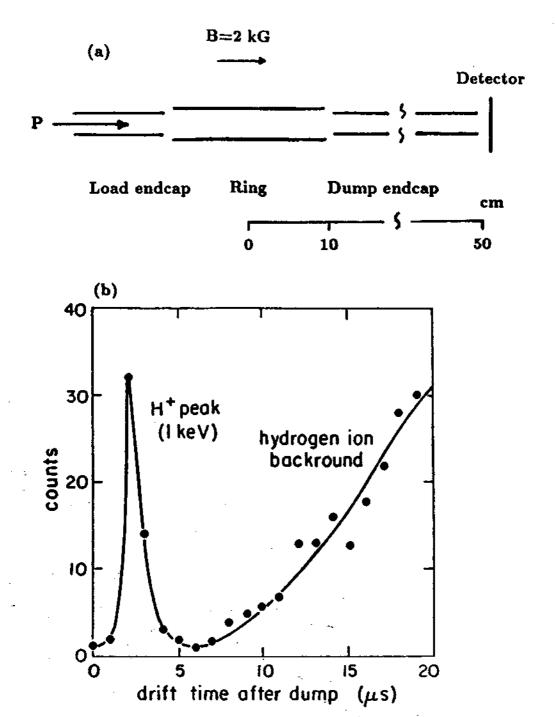
Figure 3.1: First direct trapping of keV protons.(a) Ion trap. (b) Particle counts.
