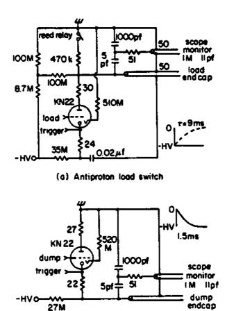
Figure 4.2: Circuit used to capture antiprotons in flight.
