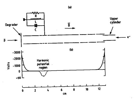
Figure 5.3: Experimental setup for antiproton slowing and cooling studies.
