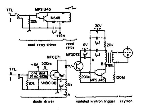
Figure 4.4: Driver circuit for the reed relay and the isolated krytron trigger circuit. The optical coupling is actually through an optical fiber. There is a misprint in Fig. 4 of the Ref.[53]. The 1  $\mu$ f capacitor between points A and B does not exist.
