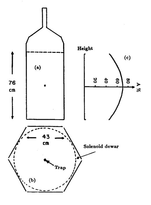
Figure 3.4: (a) Front view of a scintillator. (b) Top view of six scintillators configuration. (c) Solid angle coverage A as a function of height.
