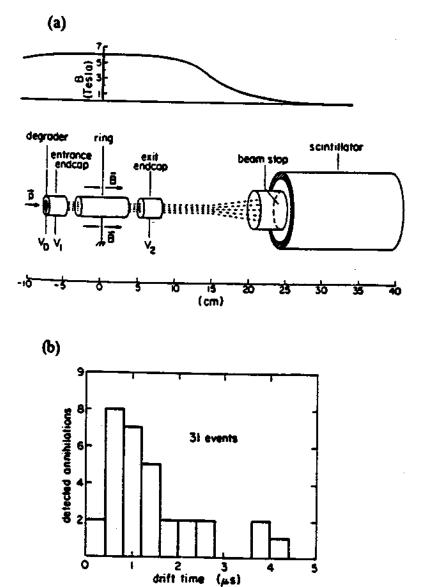
Figure 3.2: (a) Outline of the trap electrodes, the scintillator and the magnetic field. Magnetic field lines are indicated by dashed lines. (b)Time-of-flight spectrum of detected pions from antiproton annihilation.
