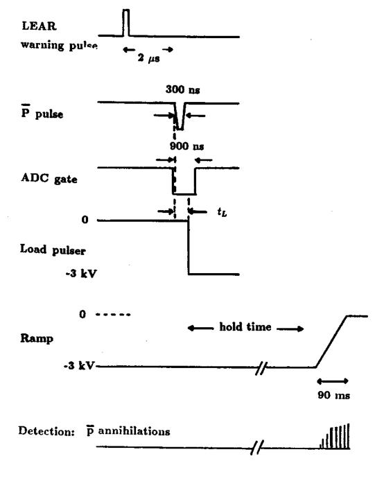
Figure 3.9: Timing sequence from LEAR warning pulse, to LEAR beam detection by PPAC, potential well switching for loading antiprotons, HV ramp to release trapped particles, and particles energy analysis.
