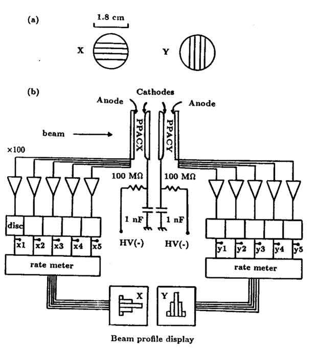
Figure 2.6: (a) The anodes of PPACX and PPACY. (b) PPAC detectors and their electronics.
