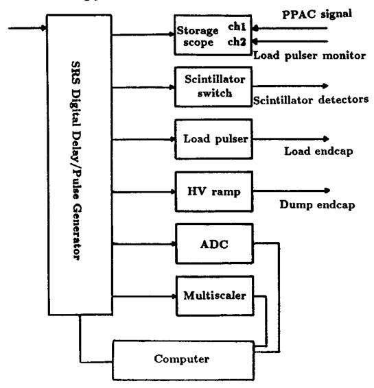
Figure 3.10: Timing block diagram
