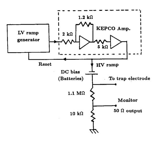
Figure 3.8: Block diagram of the high voltage ramp.
