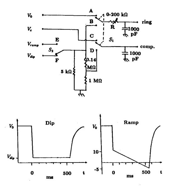
Figure 5.9: Low voltage dip/ramp circuit and its waveforms.
