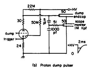
Figure 4.3: Circuit used to capture protons in flight.
