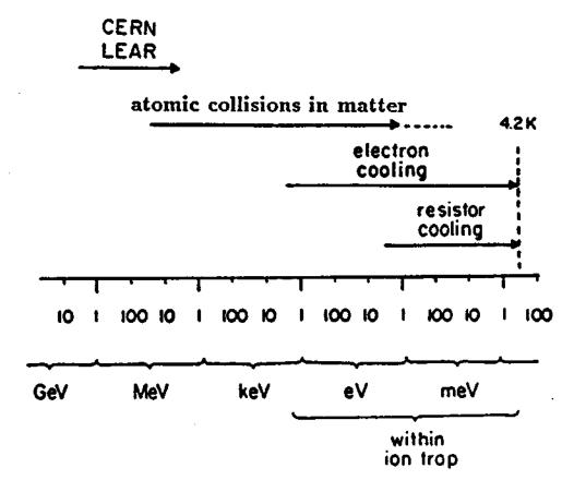
Figure 1.1: The energy span from the LEAR beam energy of about 10 MeV to the energy required for antiproton mass measurements and the methods to slow and cool antiprotons below meV.
