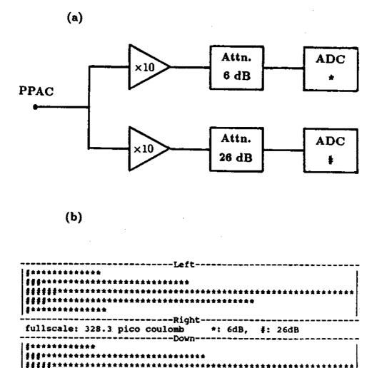
Figure 3.7: (a) Electronics for one channel of the PPACs. Other 9 are identical.
